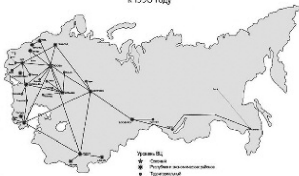
Fig. 3. Map of the basic centers of the computer centers state network (ГСВЦ) and communication lines between them (planned by 1990). Levels of centers: (1) all-state, (2) republican, (3) territorial.
